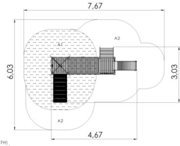
Critical fail height(CFH) A1: CFH 0.95m - 15.12m<sup>2</sup> A2: CFH 0.6m - 17.97m<sup>2</sup> Rubber surface area - 15.12m<sup>2</sup> Total area: 33.09m<sup>2</sup>
