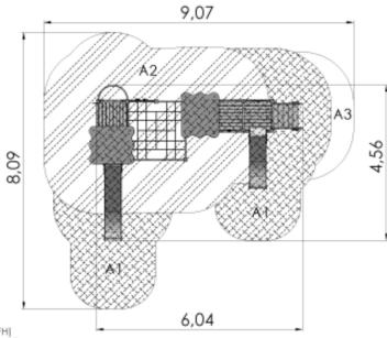
Critical fall height(CFH) A1: CFH 0,95m - 23,25m<sup>2</sup> A2: CFH 1,55m - 24,16m<sup>2</sup> A3: CFH 0,6m - 2,38m<sup>2</sup> Rubber surface area - 47,41m<sup>2</sup> Total area: 49,79m<sup>2</sup>
