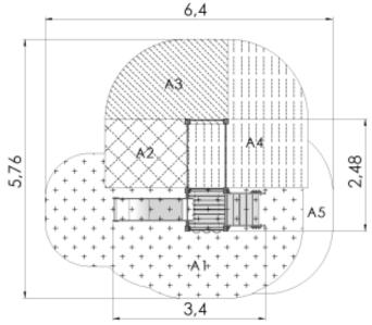
Critical fall height (CFH) A1: CFH 0,95m - 12,63m<sup>2</sup> A2: CFH 1,67m - 2,8m<sup>2</sup> A3: CFH 1,79m - 4,28m<sup>2</sup> A4: CFH 1,92m - 6,46m<sup>2</sup> A5: CFH 0,6m - 1,95m<sup>2</sup> Rubber surface area: 26,17m<sup>2</sup> Total area: 28,12m<sup>2</sup>
