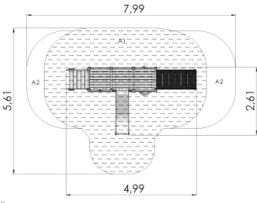
Critical fal height(CFH) A1: CFH 0,95m - 25,82m<sup>2</sup> A2: CFH 0,60m - 6,65m<sup>2</sup> Rubber surface area - 25,82m<sup>2</sup> Total area: 32,47m<sup>2</sup>
