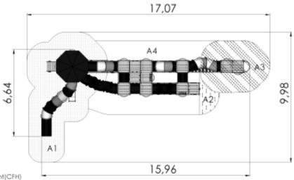
Critical fall height (CFH) A1: CFH 1.0m - 42.38m A2: CFH 1.2m - 2.64m<sup>2</sup> A3: CFH 1.55m - 17.9m<sup>3</sup> A4: CFH 0.6m - 43.54m<sup>2</sup> Rubber surface area -62,92 m<sup>2</sup> Total area: 106.46m<sup>3</sup>
