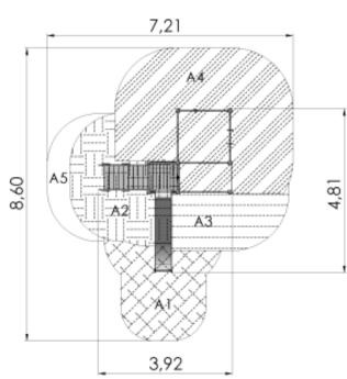
Critical fall height (CFH) A1: CFH 1,0m - 6,96m<sup>2</sup> A2: CFH 1,55m - 8,31m<sup>2</sup> A3: CFH 1,74m - 5,21m<sup>2</sup> A4: CFH 1,92m - 19m<sup>2</sup> A5: CFH 0,6m - 2,48m<sup>2</sup> Rubber surface area - 39,48m<sup>2</sup> Total area: 41,96m<sup>2</sup>
