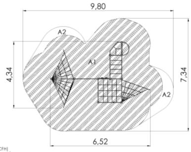
Critical fall height(CFH) A1: CFH 1,92m - 49,42m<sup>3</sup> A2: CFH 0,6m - 4,3m<sup>3</sup> Rubber surface area - 49,42m<sup>2</sup> Total area: 53,72m<sup>2</sup>
