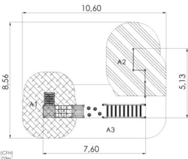
Critical fall height(CFH) A1: CFH 1.2m - 17.03m<sup>2</sup> A2: CFH 2.14m - 20.69m<sup>2</sup> A3: CFH 0.6m - 23.14m<sup>2</sup> Rubber surface area - 37,72m<sup>2</sup> Total area: 60,86m<sup>2</sup>
