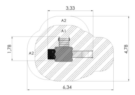
Critical fall height (CFH) A 1: CFH 0,95m - 18,64m² A 2: CFH 0,6m - 4,22m² Total area: 22,86m²
